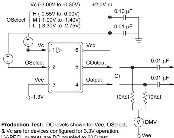
**Production Test:** DC levels shown for Vee, OSelect, &  $V_C$  are for devices configured for 3.3V operation. LV-PECL outputs are DC coupled to 50 Ω test equipment. LVDS outputs are connected to a digital volt meter, then AC coupled to the test equipment. The digital volt meter allows for Mid Level & Swing measurements.
