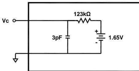
Figure 1.  $V_C$  Model – Output Enabled
