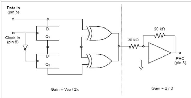
Figure 4. Simplified Phase Detector Block Diagram
