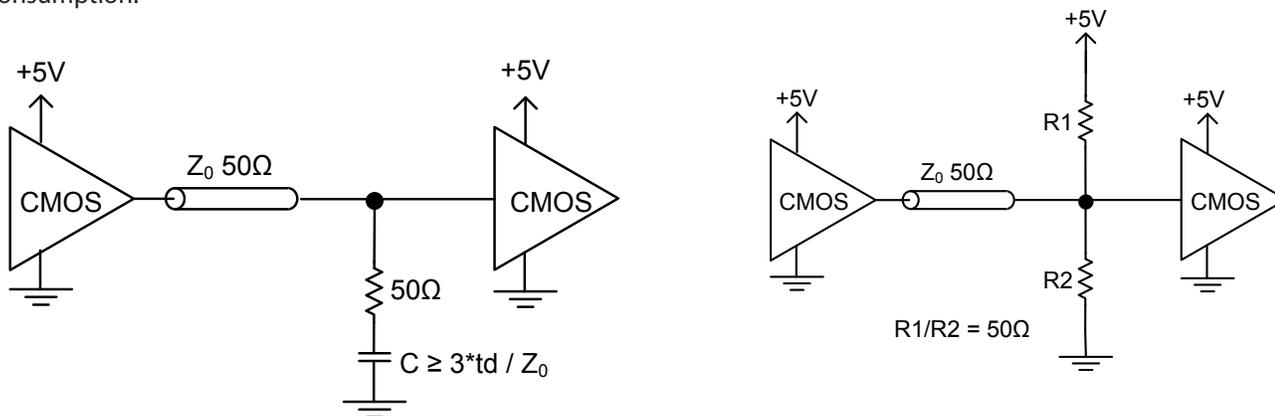
Figures 3 and 4. Alternative approaches to terminating CMOS
