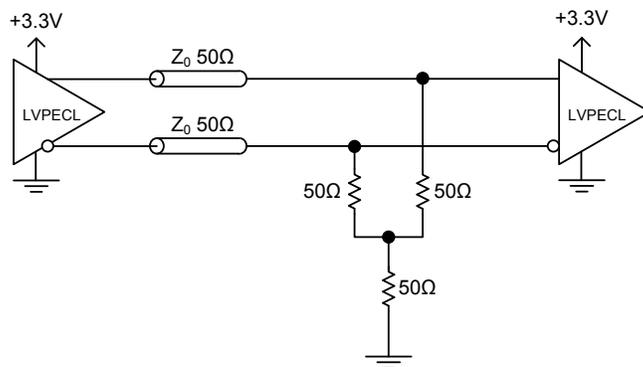
Figure 5. The most common approach to LVPECL termination
